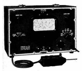
A highly stable D.C. Valve Voltmeter using an external diode probe for R.F. and A.C. measurements. Stability and freedom from zero drift are ensured by careful design and the simplified controls make for ease in handling. For A.C. mains operation, 110-120V and 200-250V, 40/100c/s.
